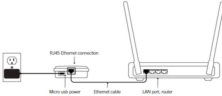
Simply connect the ethernet cable into the RJ45 port of the in.touch 2 home transmitter and in one of the available LAN ports on your router. To power up the home transmitter, plug the provided wall outlet charger to a 120V (North American model) or 220V (European model) household supply and connect the USB cable to the wall outlet and the home transmitter.
