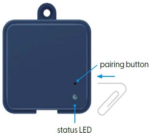
If connection issues persist, un-pairing and pairing the home transmitter may be necessary. Using a paperclip you may insert the end of the clip into the pairing button. The status LED should begin flashing yellow in a rapid pattern to show it is now in pairing mode. It will remain like this until the home module is paired or if the power is cut off to the home module.
