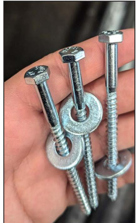
Depending on the type of spa, a piece of wood is placed on the side panels of the spa to protect it in shipping. The wooden supports are installed with several  $\frac{7}{16}$ " (11mm) bolts, once the spa is in its final resting place, remove these with an 11mm socket.
