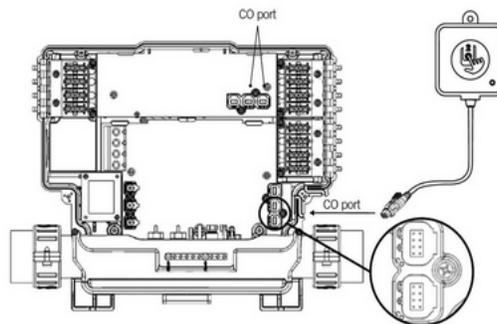
The in.touch spa transmitter must be installed under the spa skirt, at least 12" (30 cm) away from any metal component or structure, as close as possible to the house to optimize the signal strength.
